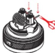
\*Ensure that the coil leads are trimmed close to prevent a short circuit. Coil leads should not touch the bell.
